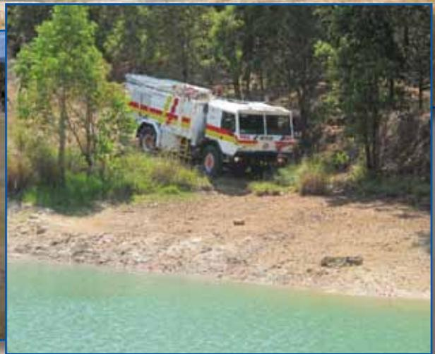
**The CAS 20- T 815-7 4x4.1 Water Tender is designed to carry a fire brigade crew (1+2) with accessories necessary for fire fighting interventions and application of water or foam using the low or high water pressure.**
