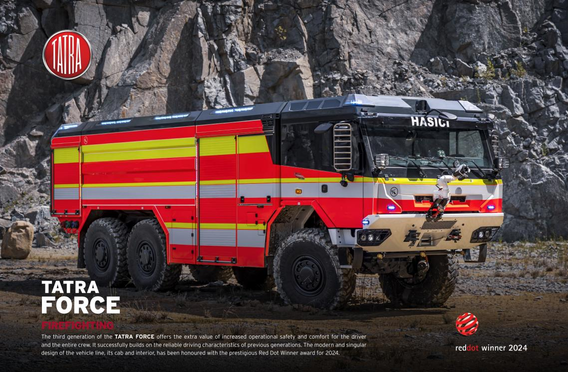
In addition to a major improvement in the existing **TATRA FORCE** concept with a low cab, engine over the front axle and a tunnel-free design, the third generation of the TATRA FORCE has expanded its portfolio to include variants with a front-mounted engine. As a new feature, the four-door cab provides above-average interior space and room for up to eight people (6 standard).
